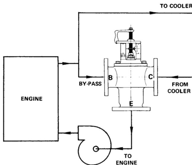
PIPING SCHEMATIC - USED AS BLENDING VALVE TO CONTROL TEMPERATURE ENTERING ENGINE.
